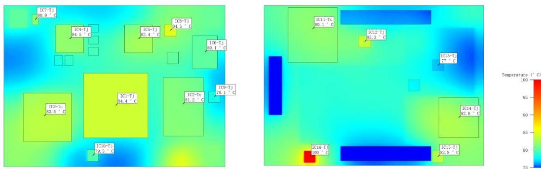
Heatsink temperature distribution contour is shown below.
